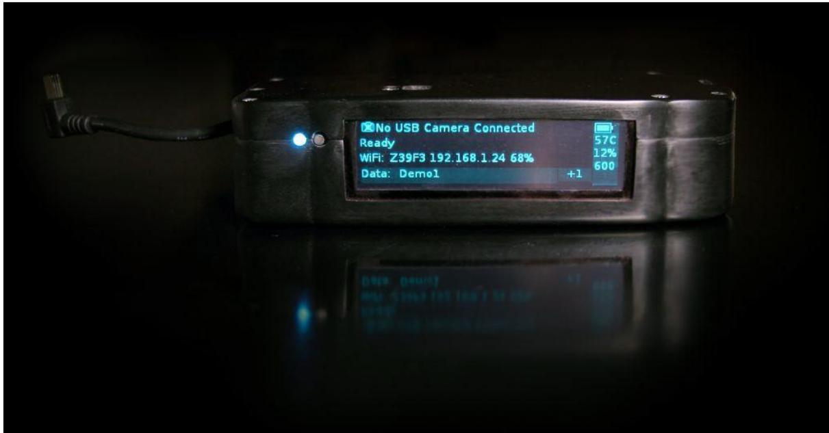
The main screen provides an overview of what the Transmitter is doing.
